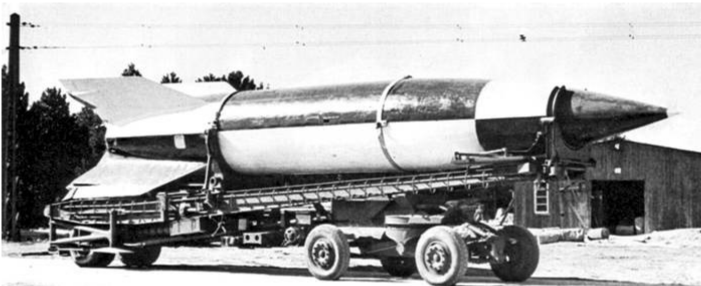
Fig. 230. A V-2 (A4) rocket on a Meillerwagen transporter vehicle. (Note: Meiller with "ll", because it was built by a company named "MEILLER", often misspelled "Meiller".)
