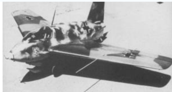
Fig. 212. The Me 163 Komet , designed by Alexander Martin Lippisch, was the only operational rocket-powered fighter aircraft during the Second World War. Although revolutionary and capable of performance unrivalled at the time, it proved ineffective as a fighter and resulted in the destruction of very few Allied aircraft—the leading edge aircraft was not very maneuverable, still not combat ready. Reitsch flew this rocket-powered aircraft on the borderline of orbital space; for all practical purposes she can easily be named as the first pilot in space or nazinaut , i.e. astronaut!
