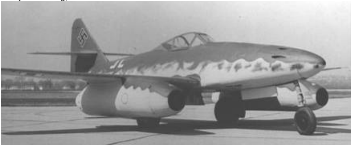
Fig. 217. Two Jumo 004 engines powered the ME 262. This was the first jet fighter to fly in combat. As a boy on the farm in Iowa, a neighbor was gunner on a B-17 bomber flying on bombing missions over Germany and occupied Europe; he had seen this Me 262 as well as the delta-wing version, which has scared the hell out of the entire crew; he never got a shot off on either one of the targets as they whizzed by at almost supersonic speeds. In WW-II, among other German military aircraft, Hanna Reitsch flew this sleek Messerschmitt 262 , which marked the beginning of modern jet aircraft flight, in fact, she was the only nazinaut and the first astronaut among her American brethren to reach the earthly edge of space, i.e. the first human in space on this planet Earth. Also, she wore her Iron Crosses proudly and wrote her memoirs, Fliegen, mein Leben (1951), which were translated in 1954 as Flying is My Life . In this book she presents herself as a patriot, and makes no moral judgments about Hitler and Nazi Germany. Fräulein Hanna Reitsch's rank was : Flugkapitän [Captain of the Air Force -- Honorary title given for outstanding aeronautical achievement].
